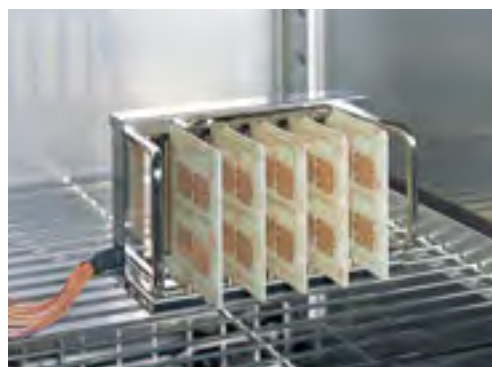
SIR test coupon type IPC-B-24 and test board rack type A (optional)
