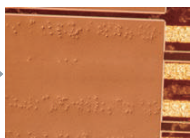
Impression of liquid crystal conductive ball, 200x [With the differential interference contrast adapter]
