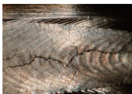
Section Fatigue Crack (50x)
