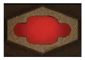
Damage to pick-up nozzles caused by cleaning is minimized. Black coating is not peeled off.
